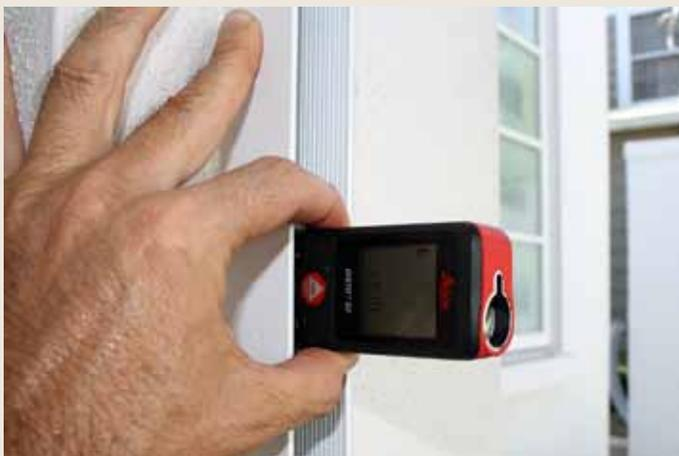
*Laser tool for measuring from inside U-channel to opposite inside U-channel*
