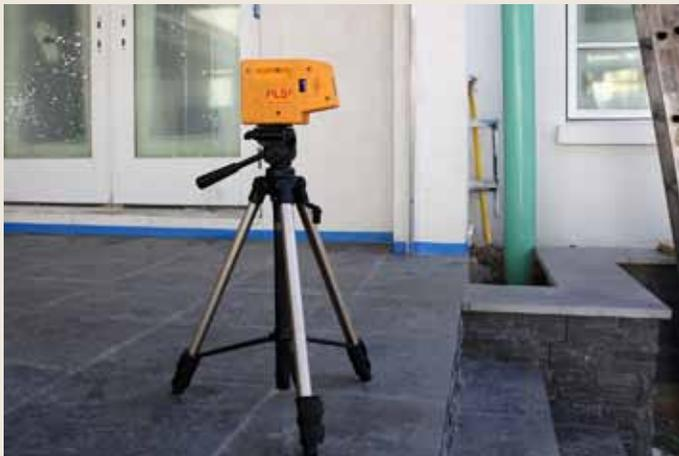
*Laser tool setup for measuring offsets*
